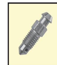
Ref: 889 607 16 Tornillo Purgador/ freno CAJA 10/Un. M 10 x 1,0 SW 11 x 30,0
